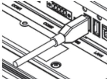
2. Insert the retaining clamp in the port above the USB connector.
