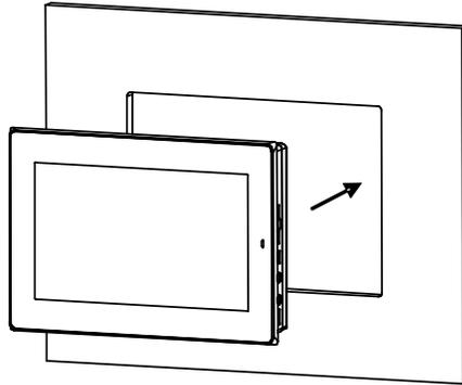
4. Insert the hook of the mounting bracket into the mounting hole as displayed in the following figure.
