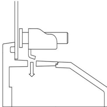
5. Tighten the screws on the mounting bracket in a clock-wise direction.
