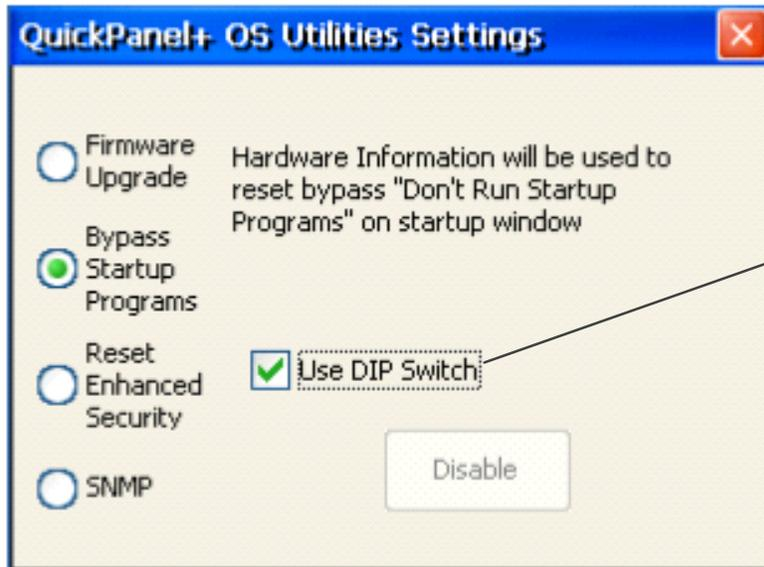
From the QuickPanel+ OS Utilities Settings window, select **Bypass Startup Programs**.
