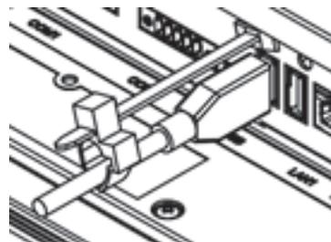
3. Adjust the position of the retaining clamp by pushing the lever of the retaining clamp. Close the retaining clamp to fit the size of the cable.
