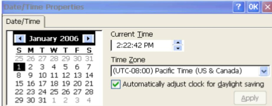
From the **Control Panel**, double-click **Date and Time** and select the date and time for the system clock.
