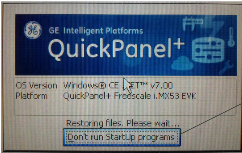
If **Disable** is double-tapped, the startup window displays . Click **Don't run Startup programs** to stop all startup programs from running .
